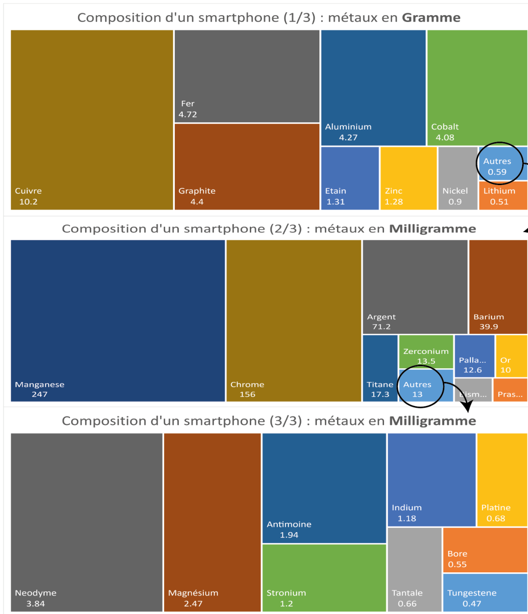
Composition of a classic smartphone, source Orange data for a Senate study 5
