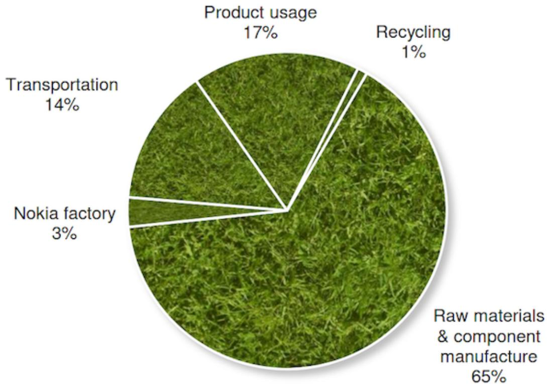
**Figure 3:** Contribution to the global warming potential of the different phases of the life cycle of a Nokia Lumia 820 **smartphone** (region of use not specified) <sup>4</sup>. It can be seen that the assembly of components by the manufacturer has a minor impact compared to the extraction of raw materials (*Raw materials*) and the manufacture of components (*Component manufacture*).
