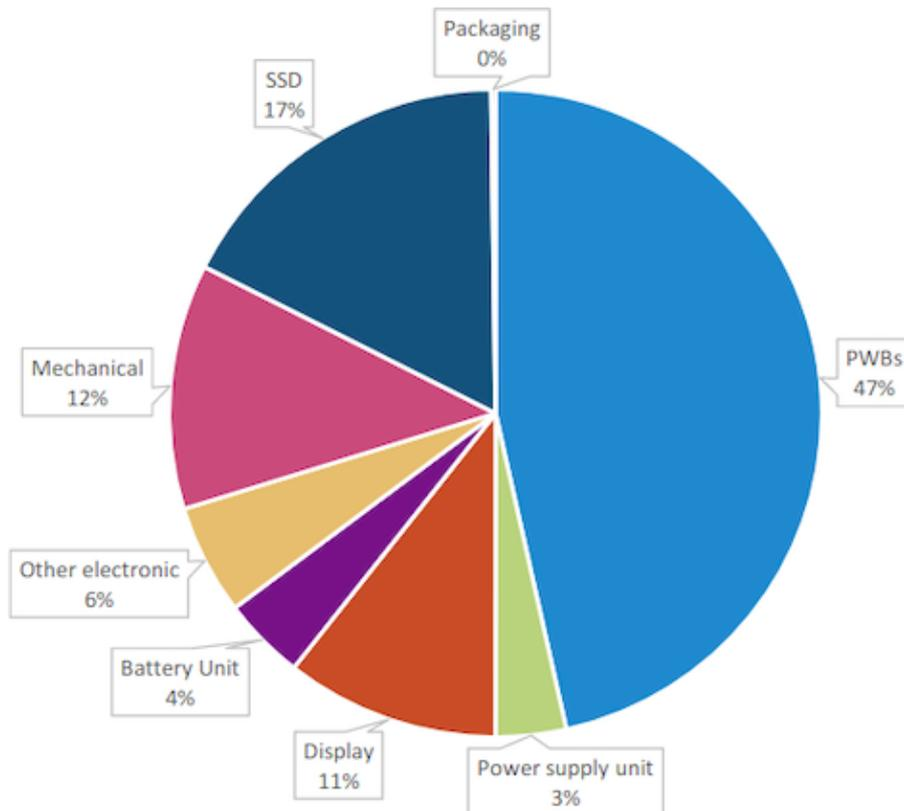
**Figure 4:** Contribution of individual components of a Dell 7300 laptop to global warming potential<sup>12</sup>. The electronic boards (*PWB*, for *Printed Wiring Board*) and the SSD hard drive are responsible for the majority of greenhouse gas emissions.
